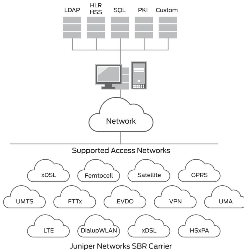
Figure 1: SBR Carrier supports a broad range of network access technologies and subscriber management data stores<sup>2</sup>
