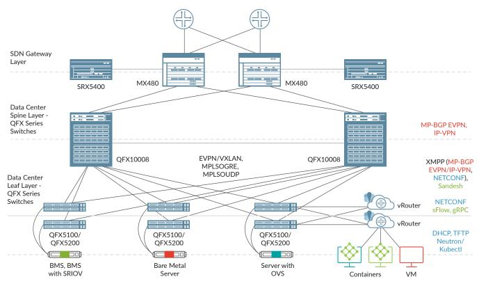
Figure 1: Contrail Networking as a fabric management and SDN overlay for data center infrastructure.
