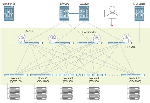
Figure 5: Virtual Chassis Fabric data center deployment with a mix of 1GbE and 10GbE
